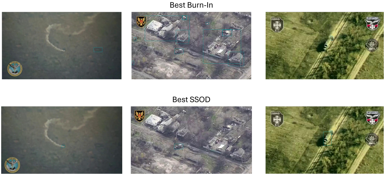
Figure 7: Some qualitative examples of predictions of the best burn-in model (i.e., without performing SSOD, top) and the best SSOD model (bottom). The bulk of the improvement for SSOD seems to come from the removal of confident false-positive predictions on background areas, most commonly square buildings or relatively high-contrast foliage. SSOD also succeeds in correctly detecting more objects that were previously missed.
