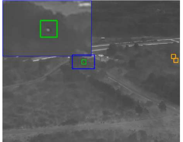
Figure 5: Frames from the evaluation dataset with detections. Blue boxes indicate the zoomed-in region shown in the top-left corner, green boxes indicate true positives, and orange boxes indicate false positives.
